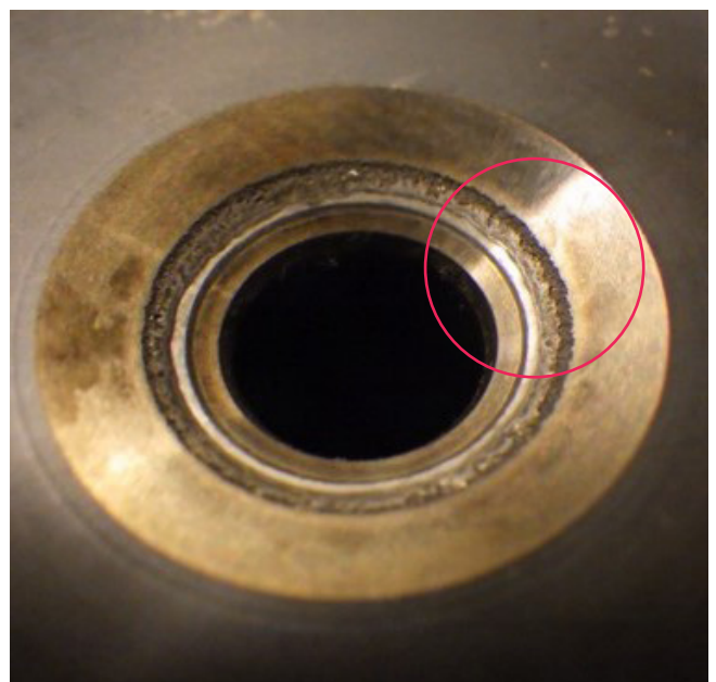
Fig. 11: Close-up of cavitation damage found at lower end of non-return valve – towards thrust spindle pipe
