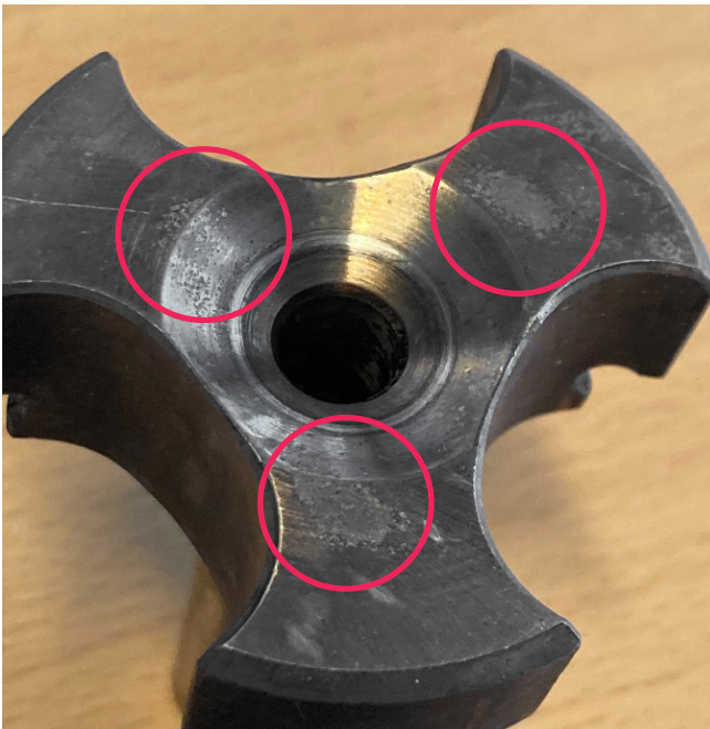
Fig. 17: Cavitation marks are considered to be merely cosmetic
