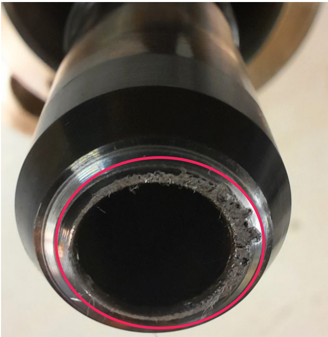
Fig. 13: Cavitation found on lower end of thrust spindle pipe – towards spindle guide
