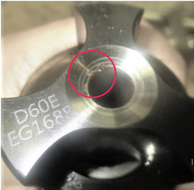
Fig. 16: Cavitation found on thrust piece in spindle guide
