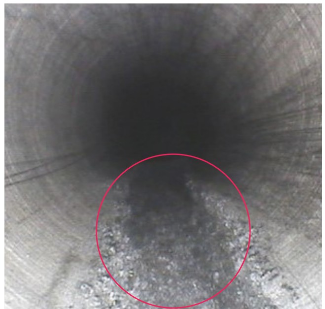
Fig. 3: An endoscope was used to inspect for damage inside the high-pressure pipe
