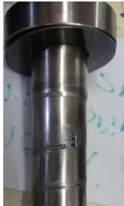
Fig. 15: Cavitation found similarly on cylindrical part of thrust spindle pipe
