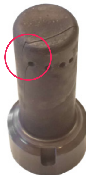
Fig. 1: Crack found on the tip of a nozzle
