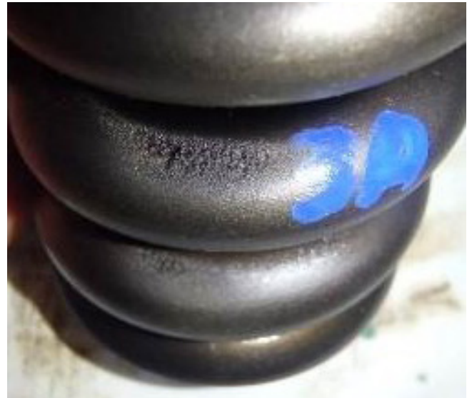
Fig. 14: Cavitation found on spring
