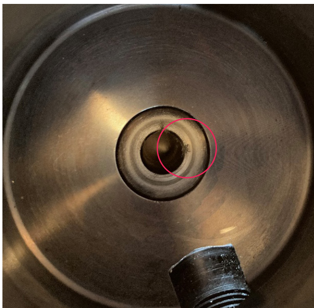
Fig. 7: Cavitation found inside fuel valve head – towards non-return valve
