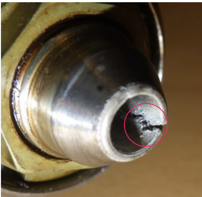
Fig. 2: Inspection of the high-pressure pipe end/seat reveals a crack – no special equipment required
